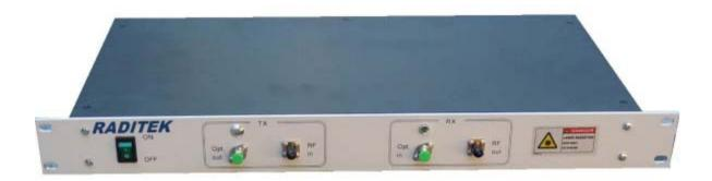
RADITEK's RF Over Fiber Transceivers can be configured one of two ways. 1) A Stand Alone One-way Transmitter and Receiver or 2) A Two-way Transceiver with Transmitter and Receiver plus a power supply in a 1 RU, 19" rack mountable shelf. The units use two optical fibers for transmitting and receiving optical signals. Tx and Rx can be combined into a single optical fiber which connects two transceivers, where signals are streaming in both directions simultaneously.
